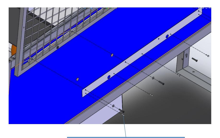
AFTER OUTTER AND INNER CLAMPS ARE LOOSELY IN PLACE FASTEN THE OUTTER CLAMP TO THE CAGE RAIL WITH #8 HEX TEK SCREWS.
