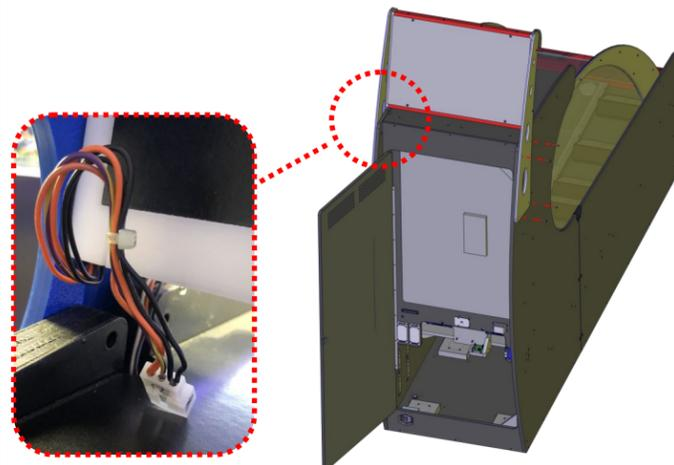
3) Carefully attach the marquee using four AA6211 Allen bolts at each side. The marquee is heavy for its size so a helper is recommended. The mating connector is located inside the cabinet shown in the diagram. Connect the harness.
