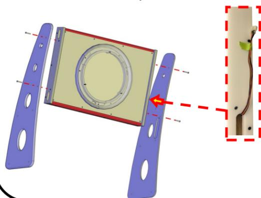
2) Open the back door. Lift the marquee assembly up onto the cabinet. Insert the marquee harness into the top hole at the left.
