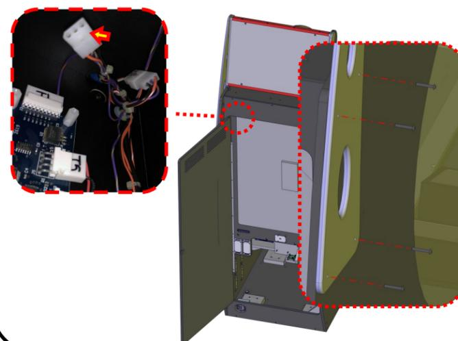
4) Install the upper wire covers onto the top sides of the cabinet using two AA6752 Allen bolts.
