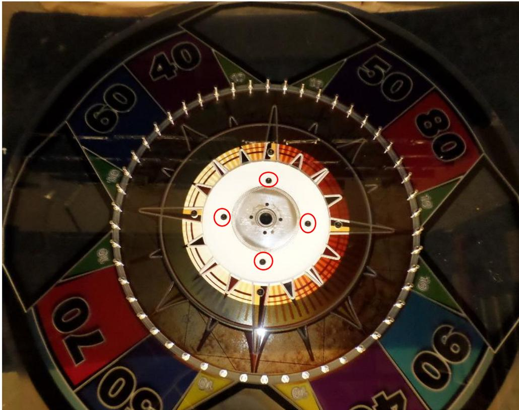
Remove the existing clutch plate from the wheel assembly, align the new clutch plate and reinstall the white inner wheel using the existing hardware.
